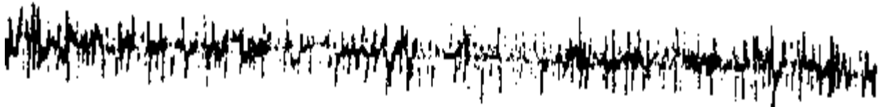
Figure 4.- Oscillogram of one-sided wear of the gear of the traction gearbox of the UZTE16M diesel locomotive: b) left rotation, 3 points.
