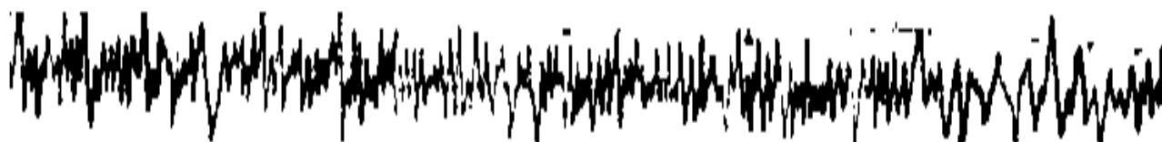
Figure 2. - Oscillogram of one-sided wear of the gear of the traction gearbox of the diesel locomotive TEP70-114, 4TED: a) right rotation, gear \frac{1}{2} , a) right rotation, UZTE16M 2 points
