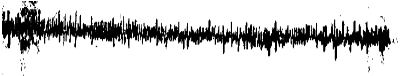
Figure 3. - Oscillogram of one-sided wear of the gear of the traction gearbox of the UZTE16M diesel locomotive:
