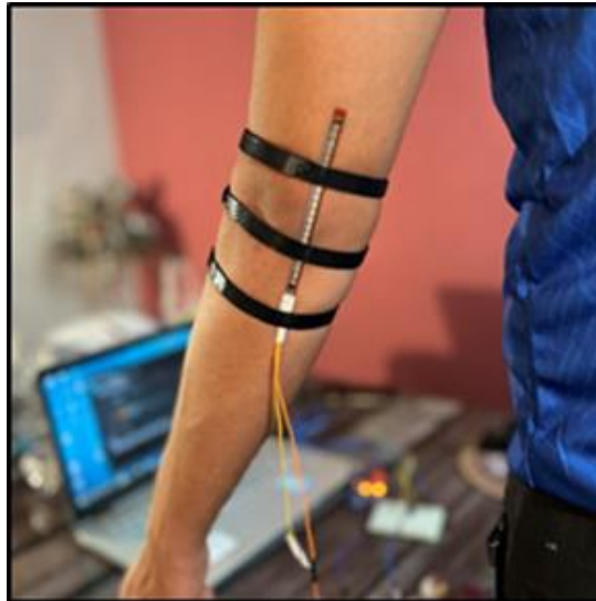
Figure 3-14: Place the Flex sensor on the biceps muscle in the extension position.
