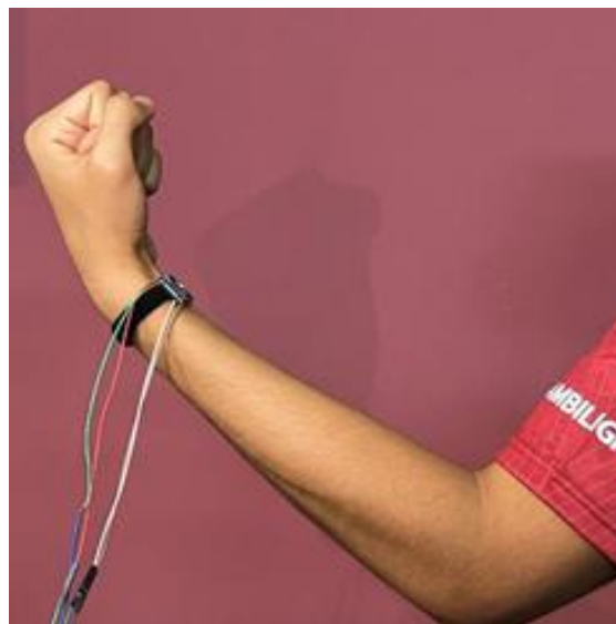
Figure 3-18: Place the Accelerometer sensor on the wrist in contraction position.
