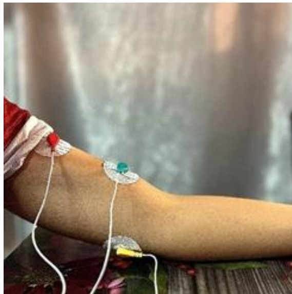
Figure 3-10: Place the EMG sensor on the biceps muscle in the extension position.
