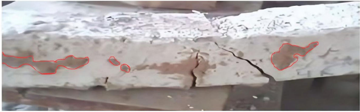
Figure 17. Beam spalling following exposure to fire [35]
