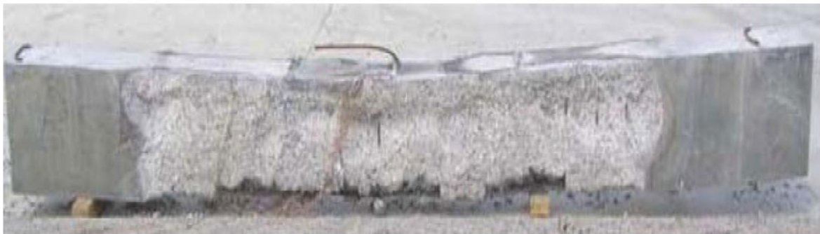
Figure 15. HPC beam spalling exposed to a prolonged fire [30]
