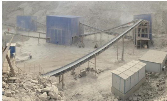
Fig. 2 Crushing plant for concrete aggregates
