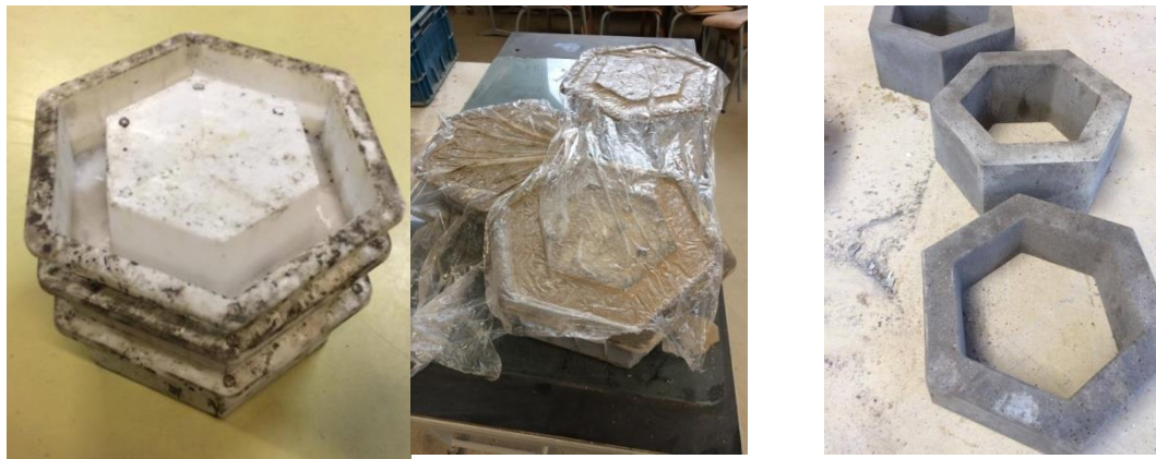
(a) Mold for concrete blocks (b) Casting concrete blocks (c) Concrete blocks after demolding
